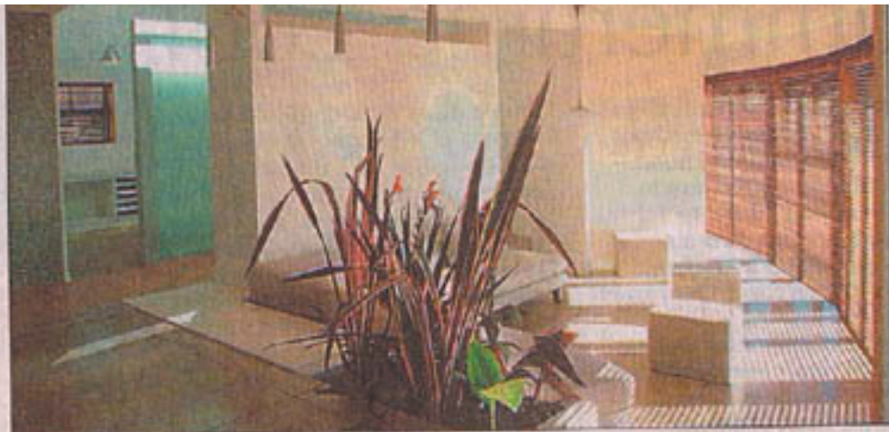
Living warmth: an internal concrete wall absorbs heat during the day and releases it at night.
